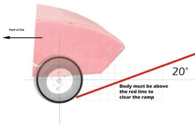
Cars will be towed up the ramp after each race, so a tow hook (eye bolt) should be provided for the tow strap. The hook must meet the clearance requirements outlined above.
