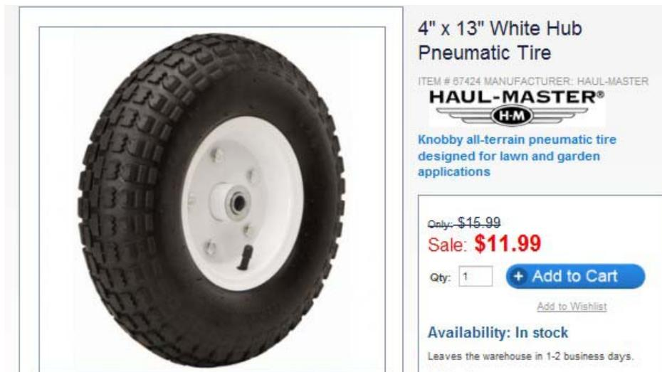
Wheels fit on a 5/8" axle. A 5/8" bolt 4-1/2" long is just the right size to go through the hub. Wheels must have some sort of locking arrangement on the nut such as a locknut or an additional nut.
